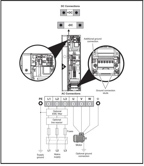
Figure 6-3 Size 5 power and ground connections
