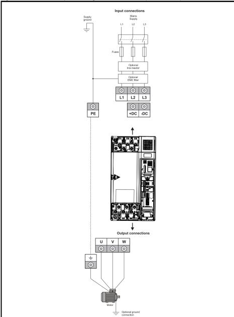
Figure 6-5 Size 7 and 8 power and ground connections (size 7 shown)
