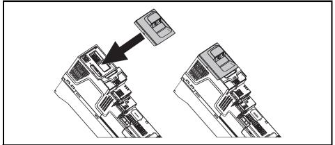
To install, align the KI-485 Adaptor and press gently in the direction shown until it clicks into position. To remove, reverse the installation instructions.
